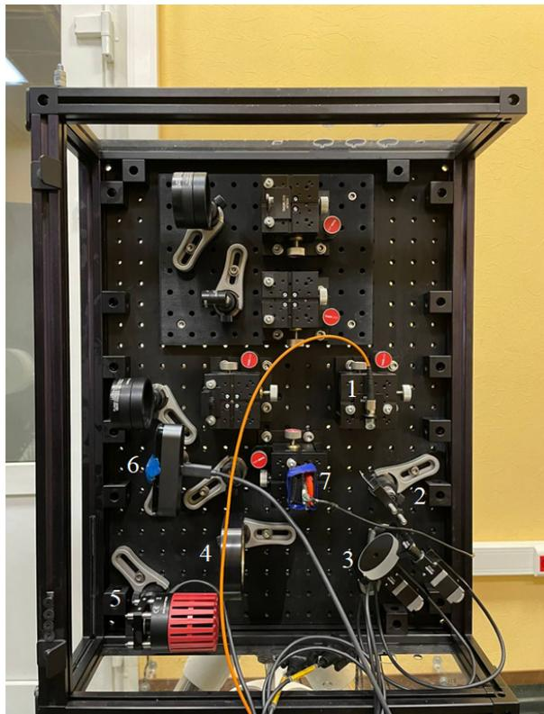
**Fig. 2.** Receiver block. Quantum channel: 1 – fiber holder, 2 – dichroic mirror, 3 – mirror, 4 – lens. Rough guidance channel: 5 – infrared LED, 6 – camera. Precision guidance channel:
