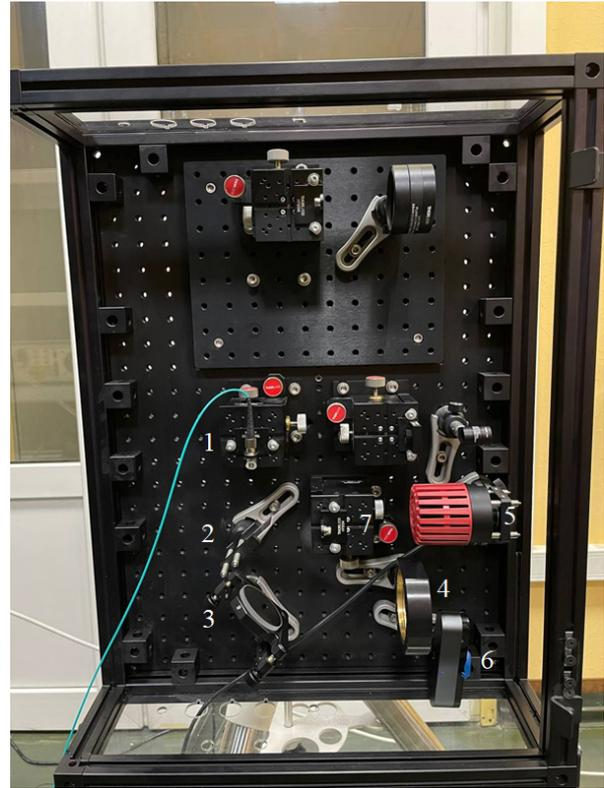
**Fig. 1.** Transmitter block. Quantum channel: 1 – fiber holder, 2 – dichroic mirror, 3 – mirror, 4 – lens. Rough guidance channel: 5 – infrared LED, 6 – camera. Precision guidance channel: 7 – fiber holder.
